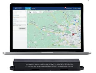
Transpoco Pulse is an ultra-low power tracking asset tracking device designed to provide seamless indoor and outdoor asset tracking on the global Sigfox network.
